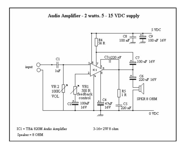
VR1 is an AF GAIN control - it controls amplifier feedback , not volume. Consequently , the *higher* the resistance value , the higher the gain ( hence volume ! )
